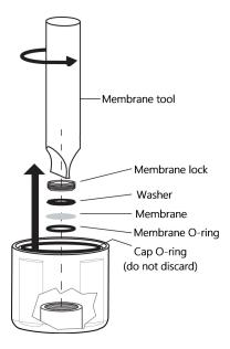
Figure 8-1. Remove membrane and membrane O-ring
