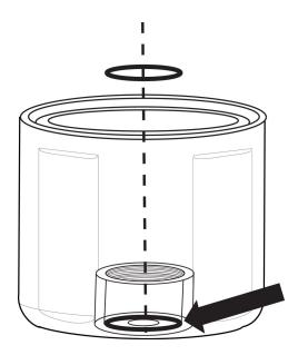
Figure 8-3. Proper O-ring placement
