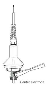
Figure 8-2. Using toothbrush to clean sensor
